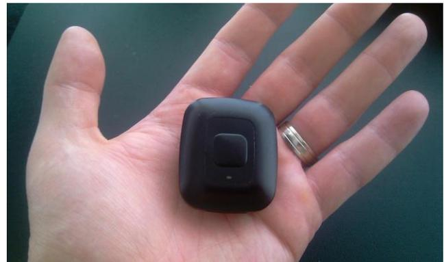
**Figure 5: Nintendo’s walk-with-me simple pedometer**
